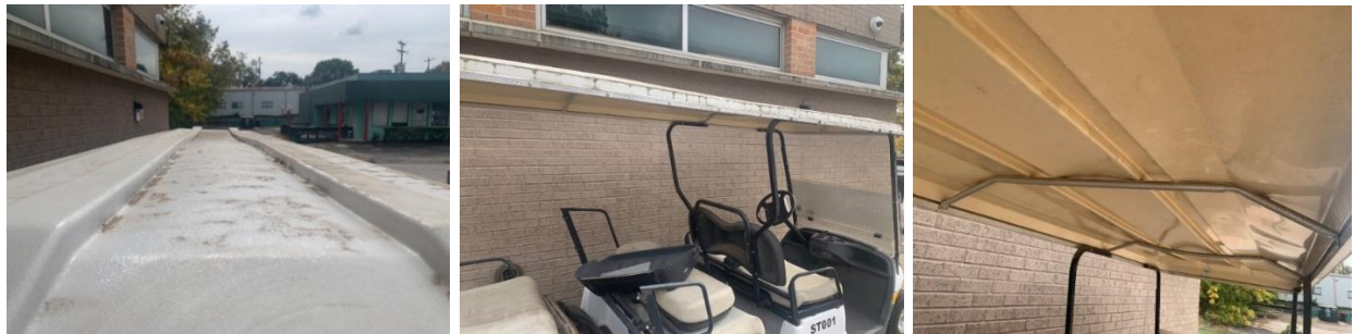
Figure 1 – a) The roof top of the golf cart, water and physical minor damages can be seen. b) The support bars on the golf cart. c) The under belly of the roof, supported by a cage to maintain its shape.
