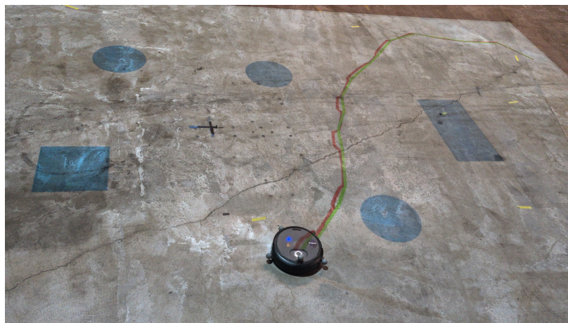
Figure 6: Robot navigation with projected paths and obstacles aligned to the physical workspace during execution.
