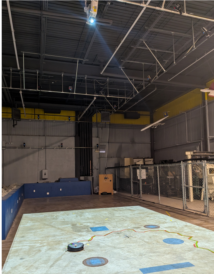
Figure 2: Experimental mixed-reality robotics testbed showing a mobile robot operating within a projected virtual environment.
