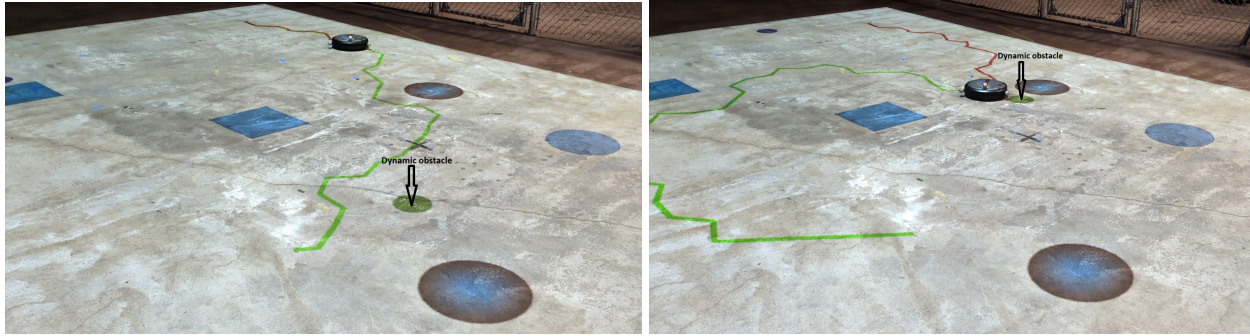
Figure 5: Real-time dynamic replanning demonstration. Static virtual obstacles are shown in blue. The green line represents the initially planned trajectory. The red path corresponds to the executed trajectory of the physical Create3 robot. In (b), a projected dynamic obstacle (labeled in the image) intersects the path, triggering online replanning
