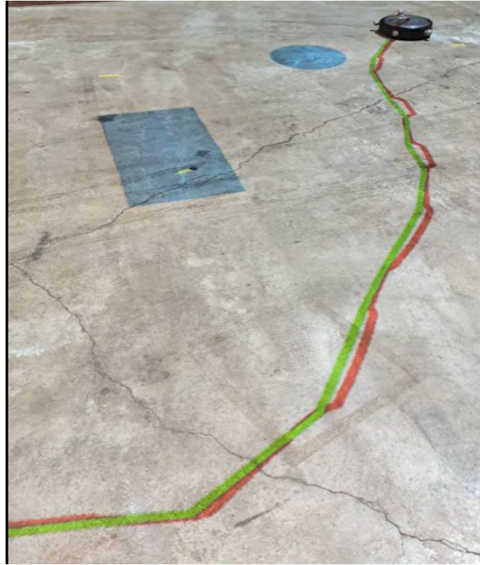
Figure 4: Comparison of projected planning results in the mixed-reality environment. Static virtual obstacles are shown in blue. The green path indicates the planned trajectory generated by the algorithm, and the red path shows the actual path executed by the Create3 robot in the physical workspace.
