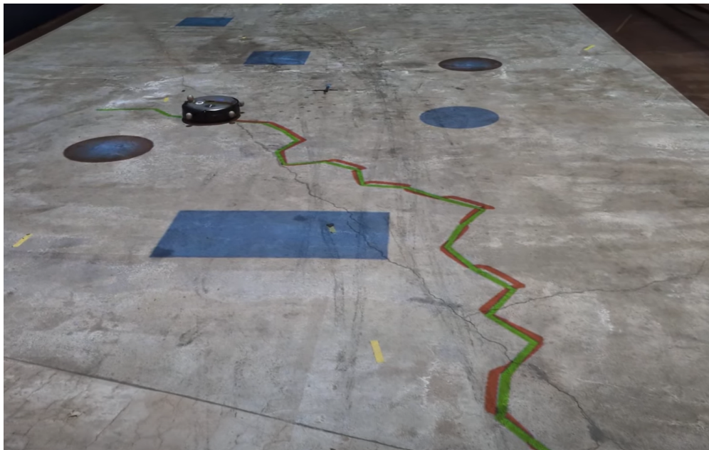
Figure 3: Mixed-reality visualization of a sampling-based motion planning solution projected onto the physical workspace. The blue shapes on the floor represent static virtual obstacles. The green trajectory denotes the planned path generated by the motion planning algorithm, while the red trajectory represents the executed path of the physical Create3 mobile robot.
