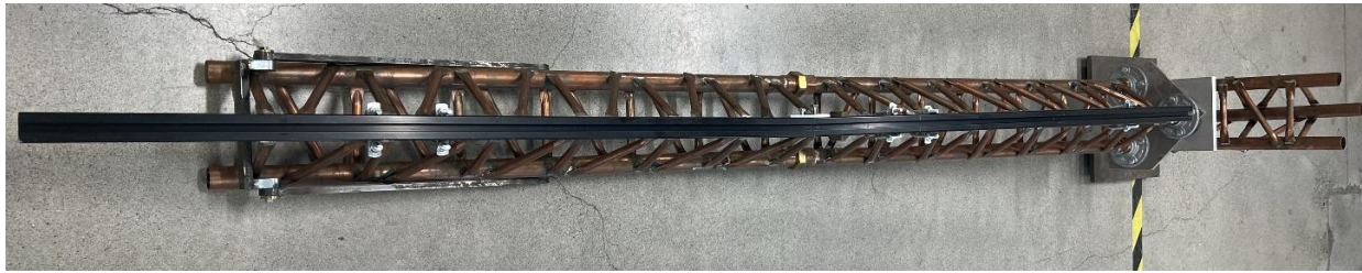
Figure 3: Picture of launch rail prototype built by ME senior design course.
