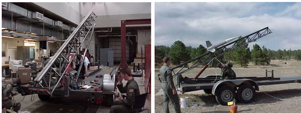
(left) Figure B2a: USAFA-built mobile rocket launcher, construction complete and installing vehicle lighting (USAFA 2002) (Right) Figure B2b: Small single-semester team rocket loaded onto USAFA mobile rocket launcher (USAFA 2002)
