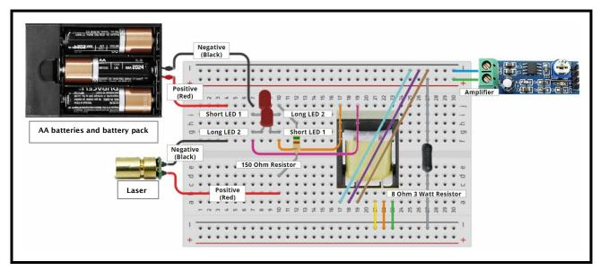
Example image from manual showing wired connections on solderless breadboard and components
