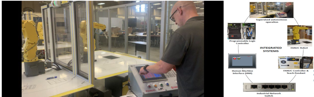
Figure 5: Development of training system using Fanuc Integrated with PLC and HMI
