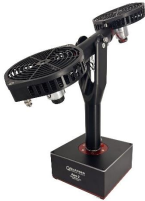
a) 1-DOF VTOL (Vertical Take Of Landing), Half-quadrotor.
