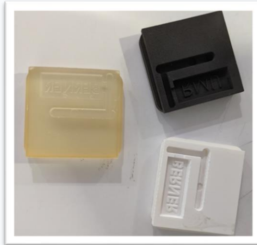
Figure 7. SLA and SLS printed mold inserts
