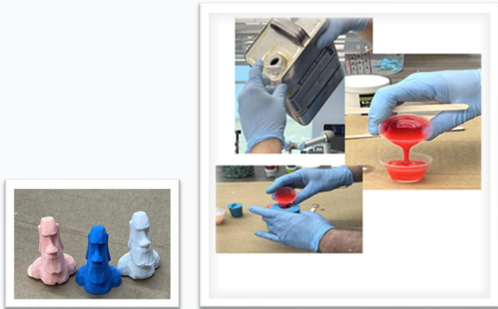
Figure 11. a) FDM/FFF printed pattern (dark blue), molded pieces (light-pink and -blue) b, c, d) Pouring the resin into silicone rubber mold
