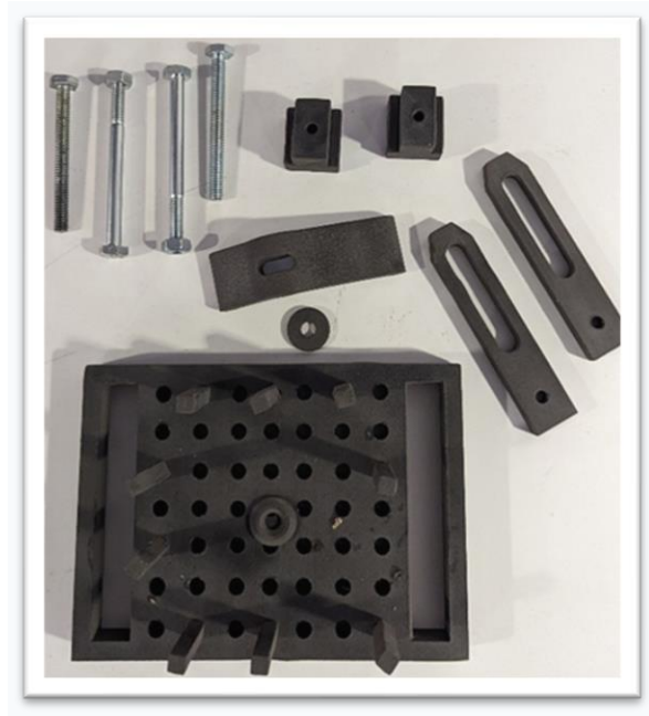
Figure 14. Completed machining fixture -printed mainly by SLS by the participants.
