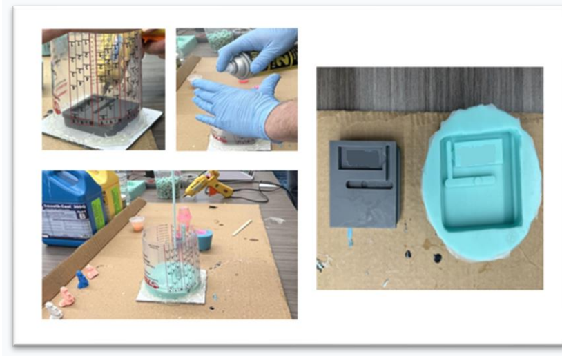
Figure 9. a) Preparation of the mold by introducing a cover to the SLA printed mold insert b) Application of a mold release agent c) Application of the silicone rubber mold mix (with parts A and B) d. Initial (grey) negative and resulting (green) positive tooling.
