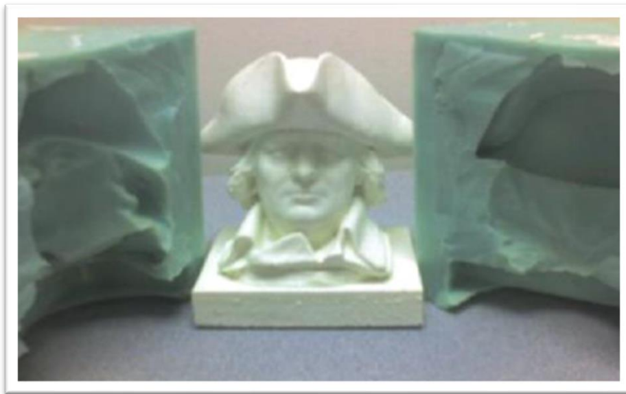
Figure 7. RTV mold halves and resulting polyurethane replica
