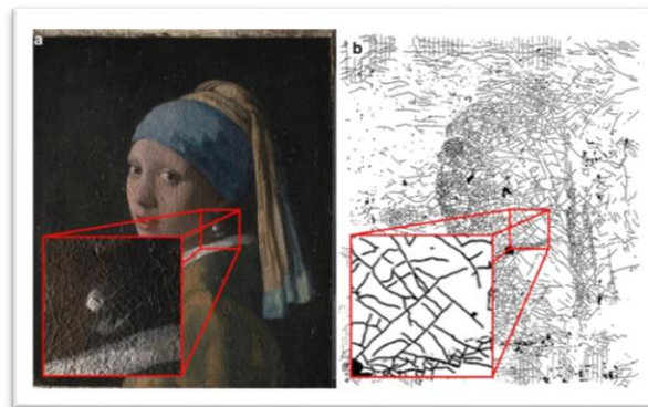
Figure 1. RLP studies painting and its cracking patterns, documented by manually tracing the cracks onto a transparent polyester film [8]
