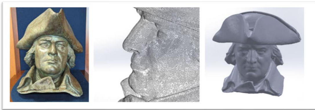
Figure 5. a) The bust after its restoration b) Polygon file c) Resulting STL
