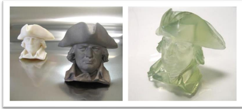
Figure 6 a) FDM- b) Prometal- c) SLA-printed replicas
