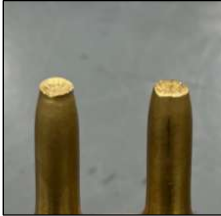
Figure 17. Necking Pattern Characteristics
