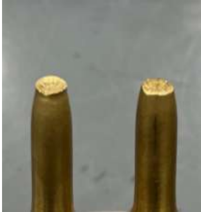
Figure 2. Necking Pattern Characteristics
