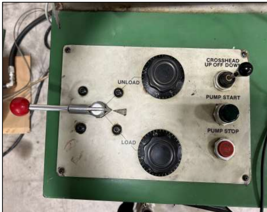
Figure 9. Test Controls on the TTM Control Box
