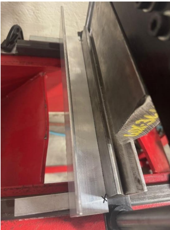
Figure 5. First L beam for 1 st bend on left side of punch
