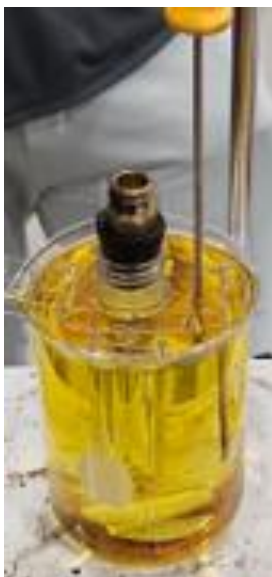
Figure 9. Submerging preform in antifreeze up to neck ring
