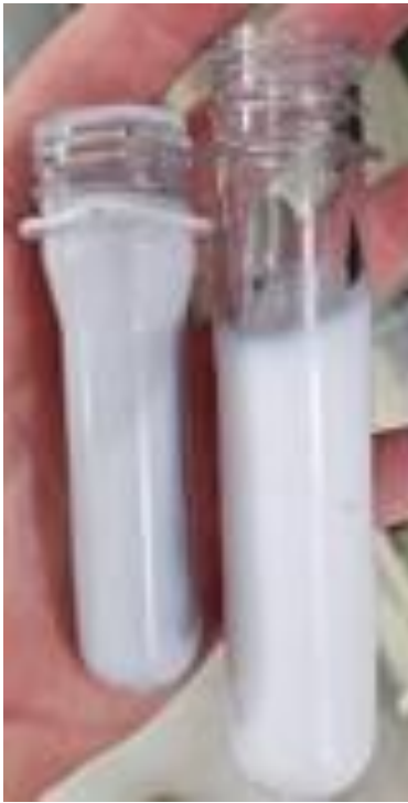
Figure 12 Examples of over-heated preforms
