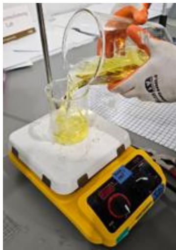
Figure 5 Filling beaker with antifreeze
