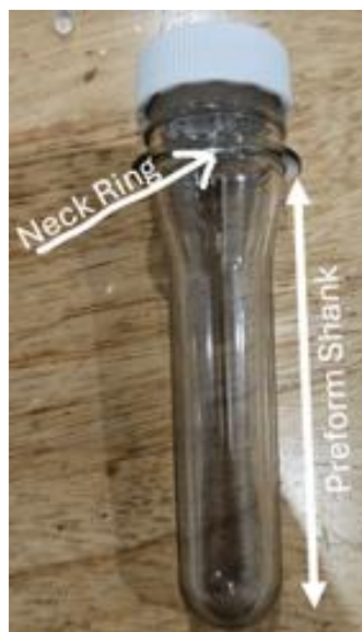
Figure 9. Submerging preform in antifreeze up to neck ring
