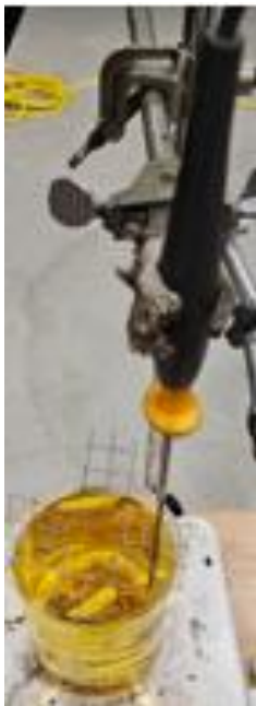
Figure 7. Thermocouple thermometer probe in antifreeze
