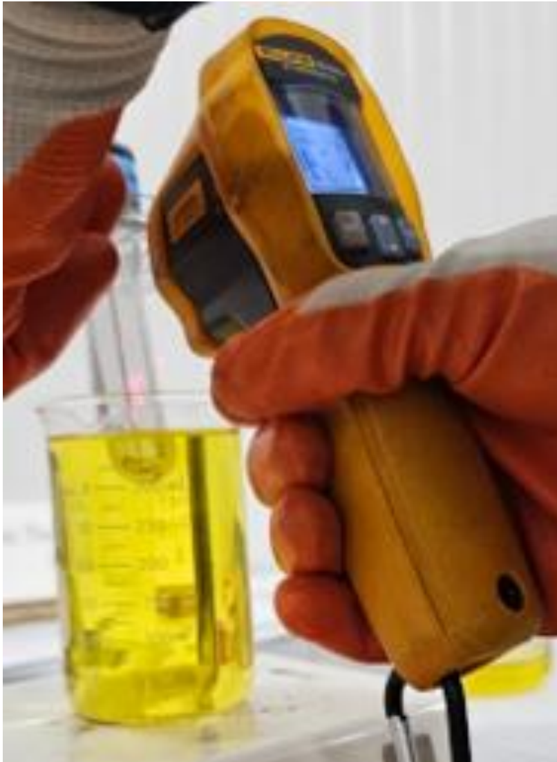
Figure 10. Measuring temperature of preform
