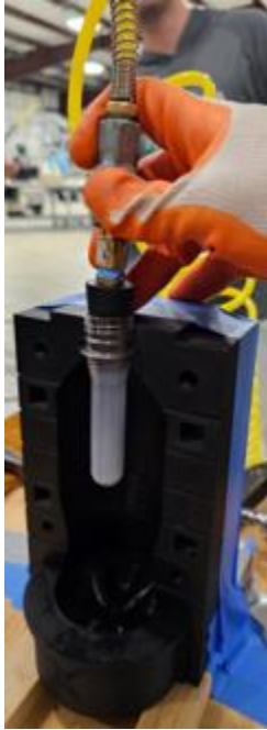
Figure 1a) Section View of Preform in Mold
