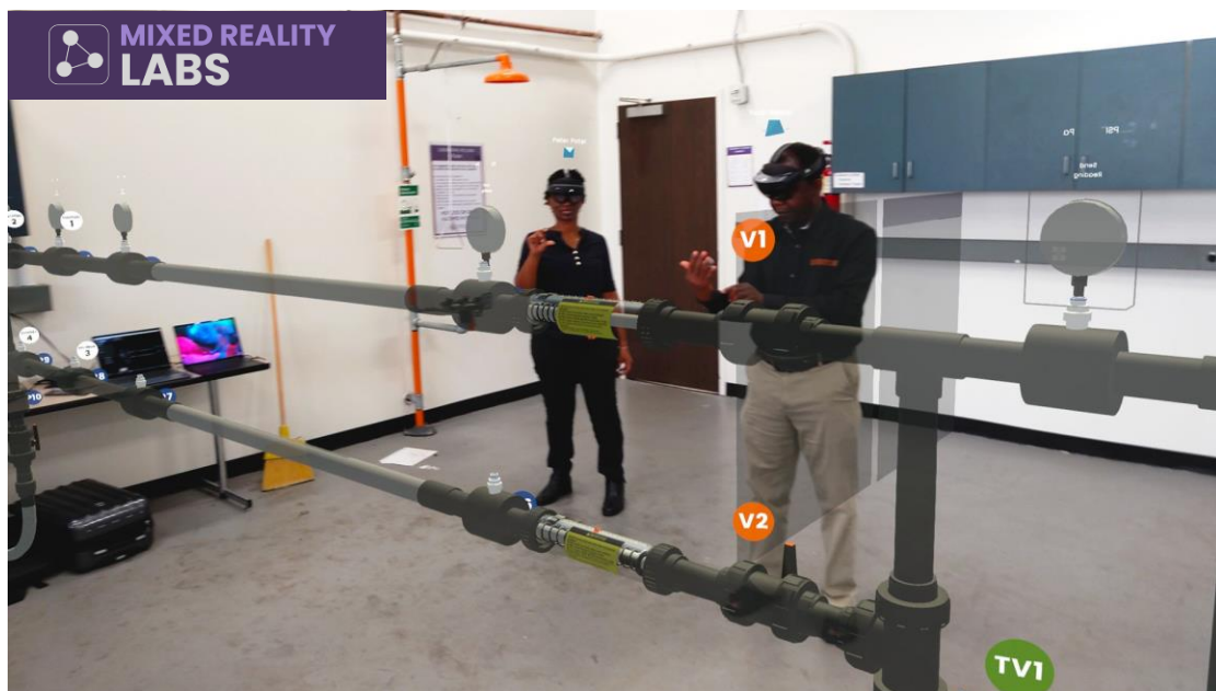
Figure 5. Two members of the project team testing a working MR digital twin of the fluids mechanics equipment.
