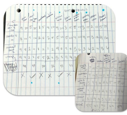
Fig. 3. (a) Examples of ideation, decomposition, clustering, and morphing (b) and Pugh screening and scoring.
