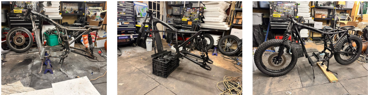
Appendix 5. Frame preparation and paint application.
