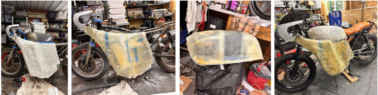
Appendix 8. Fairing and tank construction.
