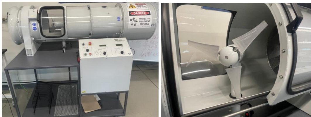
Figure 6 The AE1005V Wind Turbine Dynamics module and the control panel are shown on the left. The figure on the right shows a close look of the 3D-printed blades installed on the turbine hub. The glass window is closed during the operation.
