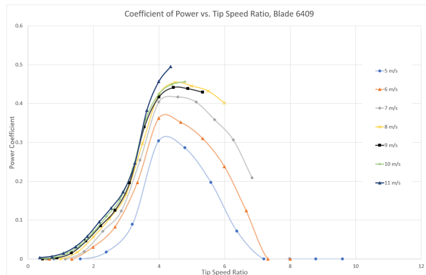
Figure 8 An experiment done to map the C_p vs. TSR graph for Blade NACA6409 at varying windspeeds. Notice that the peak for all windspeeds lies at a TSR of about 4.3 and a C_p ranging from .32 to .5 at zero yaw and pitch of 5 degrees.
