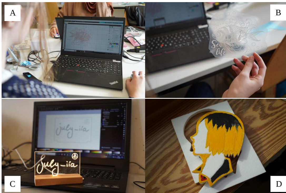
Figure 1 Pictures of P12-activity examples at H-BRS: A) technical drawing with Silhouette Studio with B) resulting folio-cut, C) laser-cut example with CAD file and D) hot-wire foam cutting example
