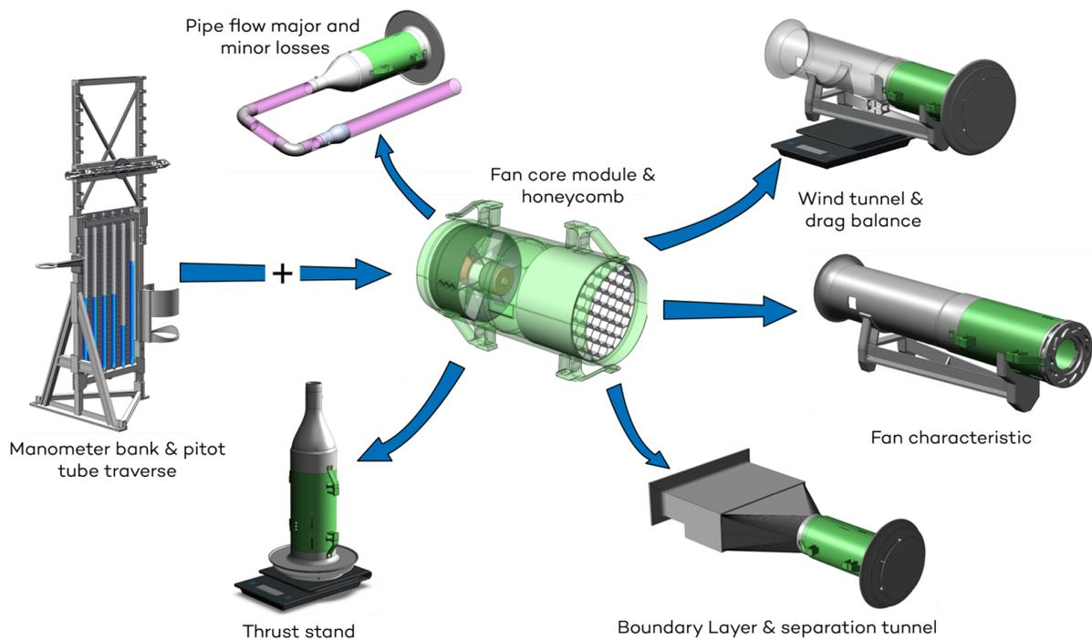
*Figure 3: Experiment Options for the Fan Core Module.*
