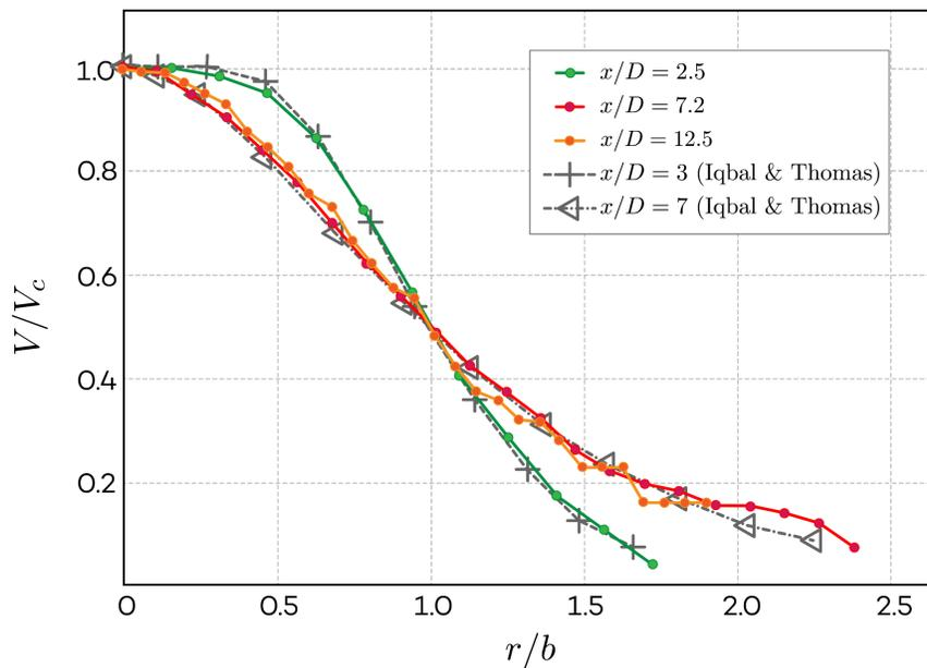
Figure 7: Comparison of normalized velocity profiles to Iqbal & Thomas [8], with  $V_c$  being the centerline velocity of the profile, and  $b$  is the radial position where  $V/V_c = 0.5$ .
