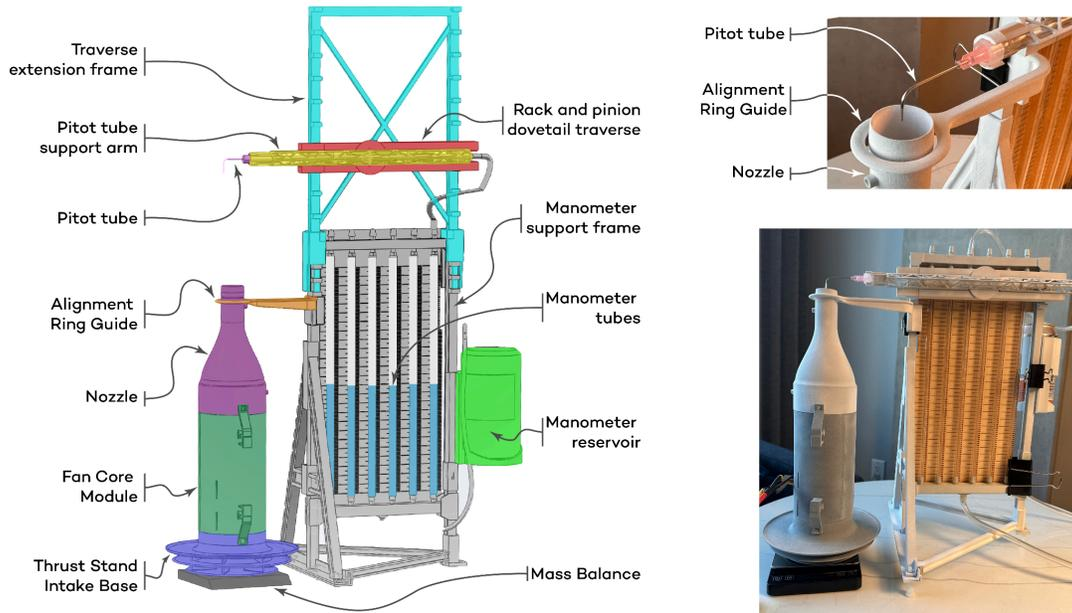
Figure 4. Assembled manometer bank and traverse mechanism, showing guide ring and traverse extension. b) close up image of nozzle exit and ring guide, along with pitot tube. c) detail of traverse extension and
