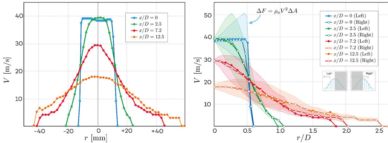
Figure 6: (left) Radial velocity profiles at four downstream stations ( $x/D = 0, 2.5, 7.2,$  and  $12.5$ ) shown across the full span. Note that the traverse limit prevented measurement at locations  $r < -40$  mm. (right) Radial velocity profiles with the left-side profiles mirrored across the centerline, and corresponding force contribution  $\Delta F = \rho_a V^2 \Delta A$ .
