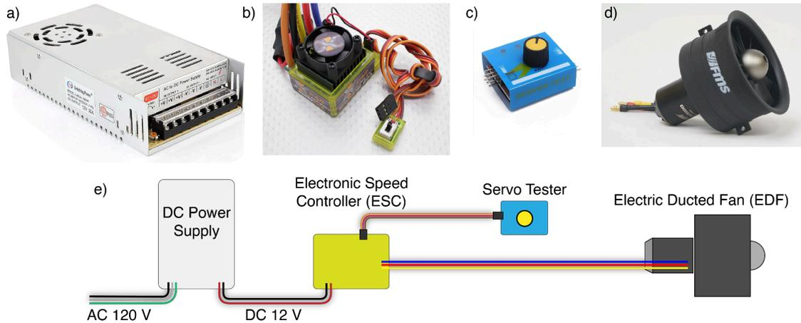
Figure 1: a) DC Power Supply, b) Electronic Speed Controller (ESC), c) Servo Tester to provide fan speed signal, d) 64 mm diameter Electric Ducted Fan (EDF), and e) wiring connection schematic.
