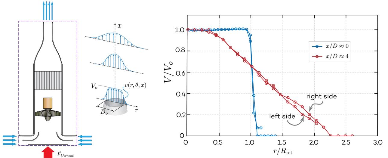
Figure 5: Thrust stand control volume for momentum flux calculation (left). Radial velocity profiles at two downstream stations using research-grade pitot tube and manometer (right).
