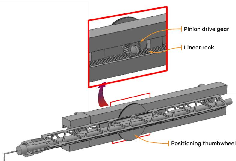
Figure 5: Detail of dovetail traverse with rack and pinion positioning. The gear ratio is such that one revolution of the thumbwheel moves 32 mm. The wheel is marked with divisions that permit reliable positioning at 1 mm increments. Total range of the traverse is 100 mm.
