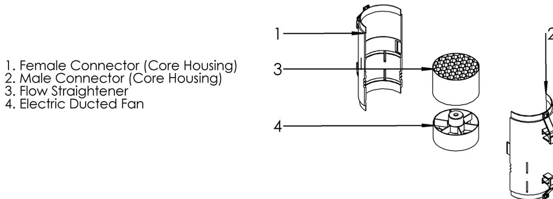
Figure 2: Exploded View of the Fan Core Module.
