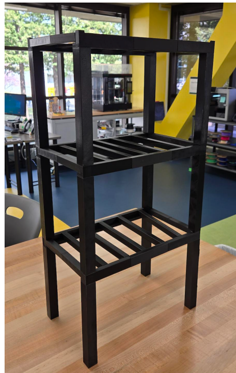
Figure 2. Photo of the assembled Load Path Explorer prototype showing its modular structural components.
