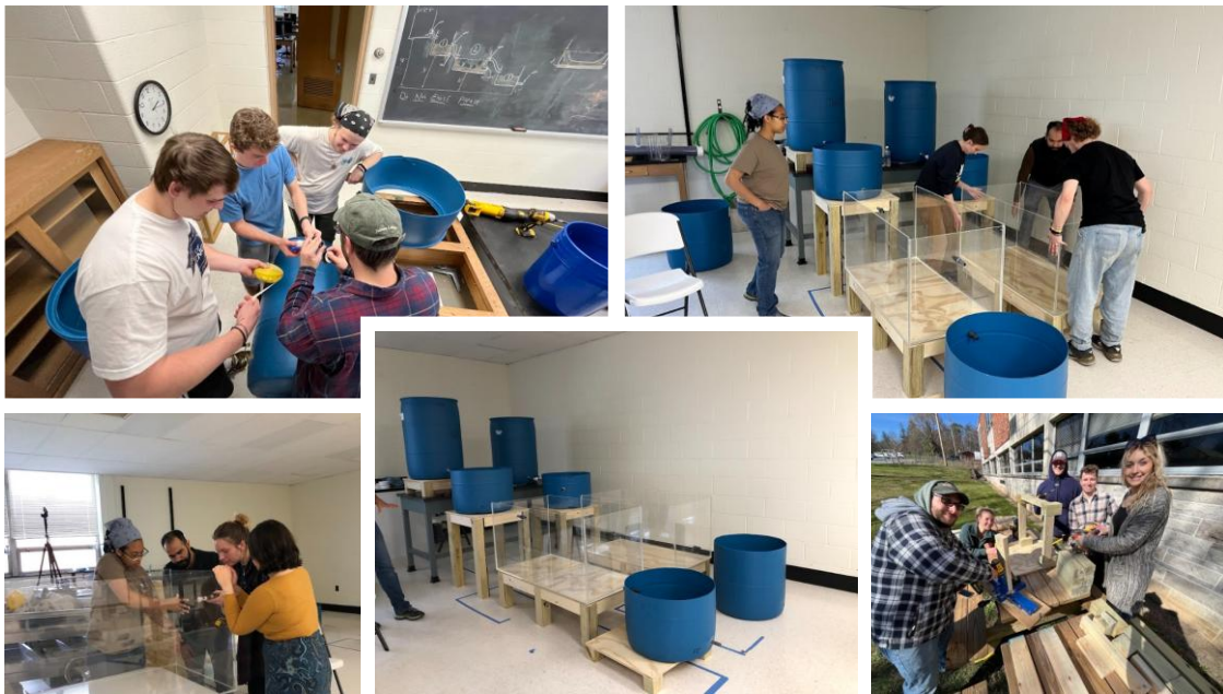
Figure 4: Group of students building platform and tanks for wetland
