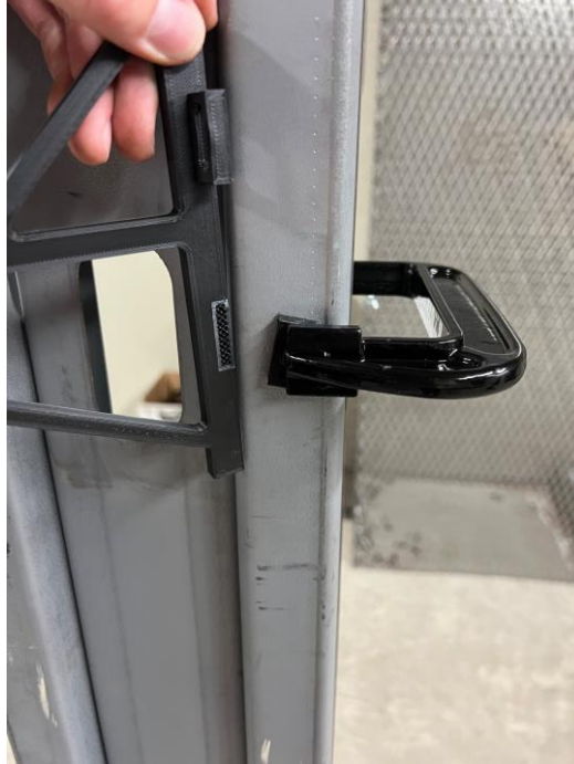
Figure 13: Test 1 Mounting Tab Failure.
