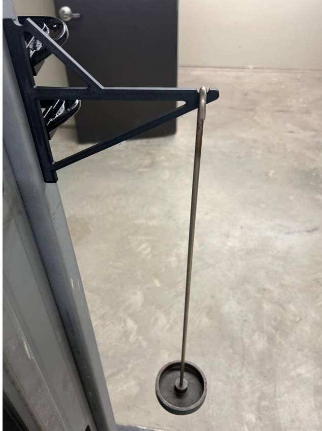
Figure 12: Clamped Bracket (V3) with hanger off the end.
