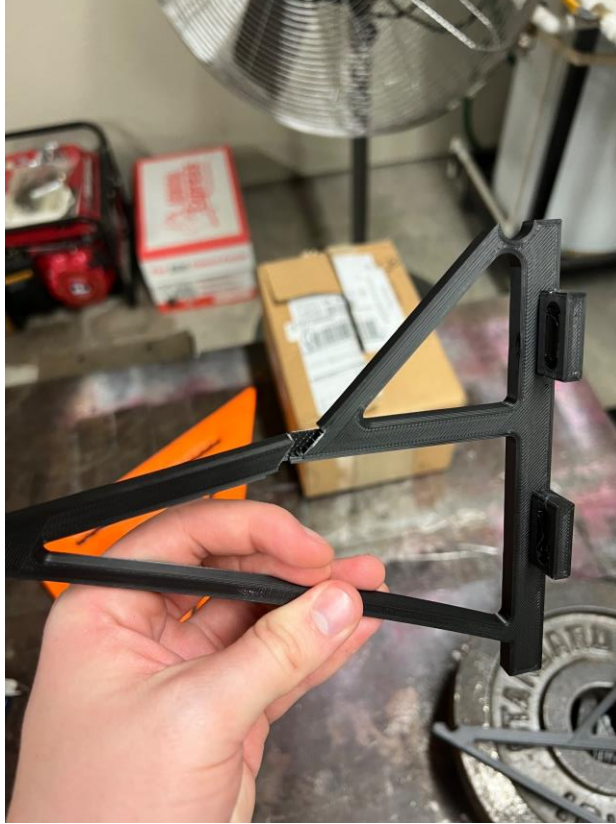
Figure 14: Test 2 Central Intersection Failure.
