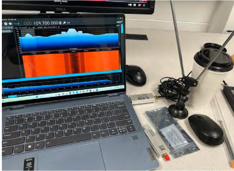
(a) Basic setup for listening to FM Broadcasting at SDRSharp using RTL SDR
