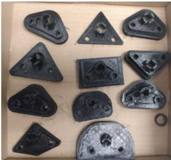
Figure 6: 3D printed visor brackets designed by students
