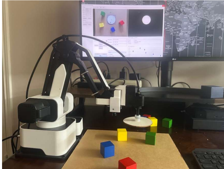
Figure 7 The air picker picks up the identified object (round coaster blank)
