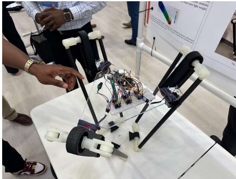
Figure 8 Prototype of a Delta robot
