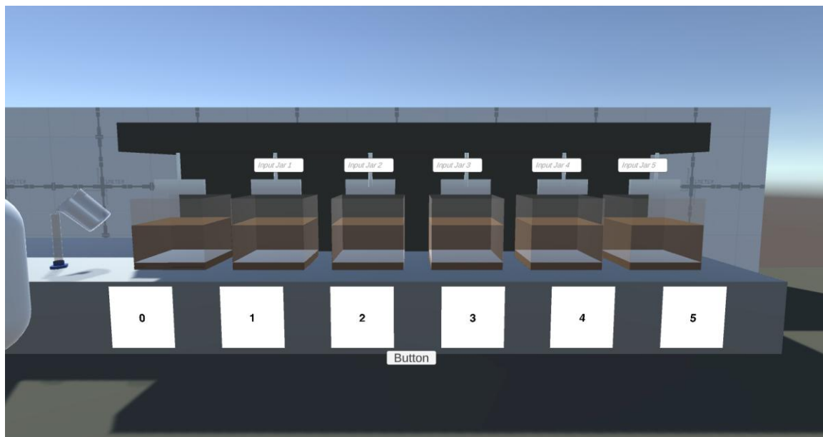
Figure 1: The jar testing apparatus from the Unity Jar Test as shown while selecting the input parameters. After selecting the button at the bottom of the screen a time-accelerated animation will play depicting the process.
