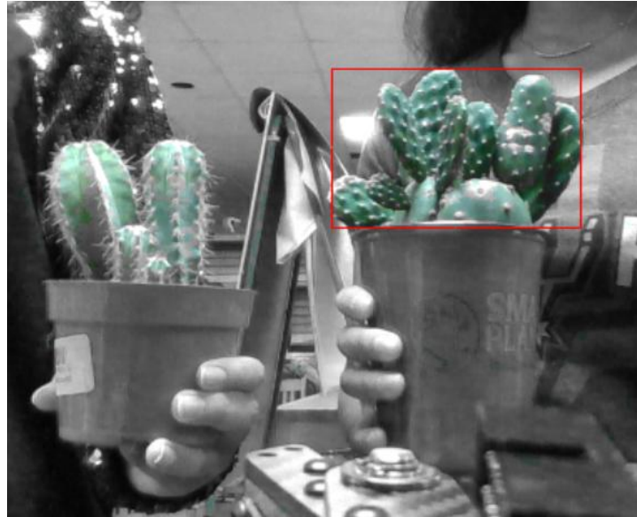
Figure 5. Proof of Concept – Red box indicates the QArm identifying the specific color of the Prickly Pear Cactus (Hue 147.6°)
