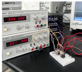
Source Voltage DC P/S connected to +ve terminal in a voltage divider configuration
