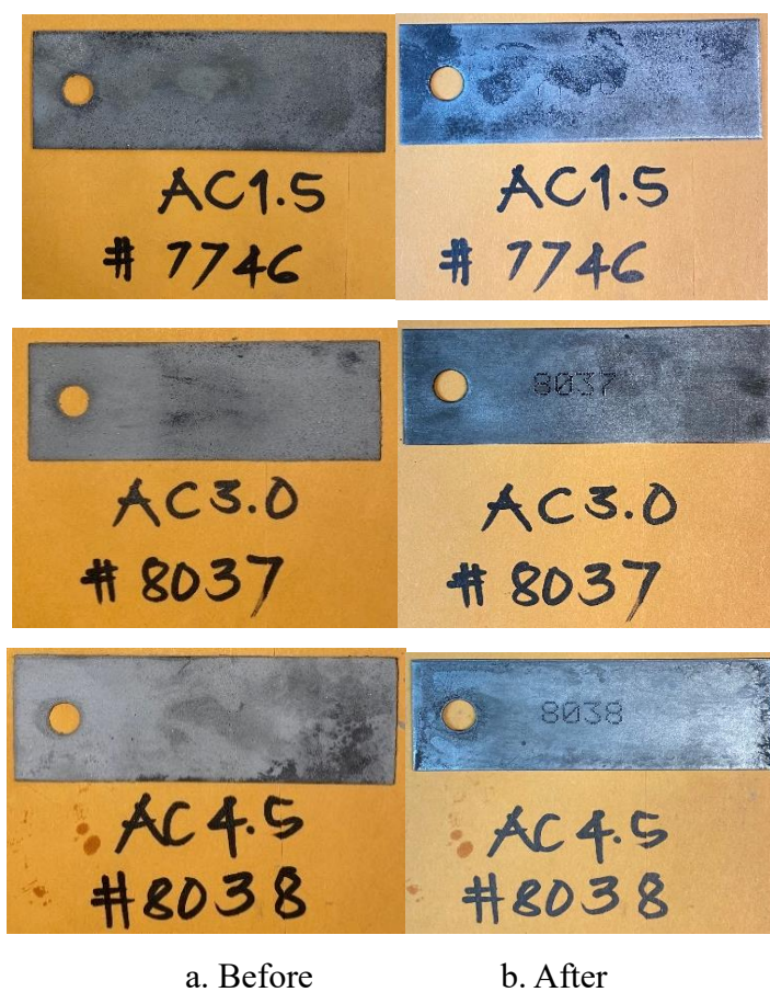
Figure 4. Corrosion plates in potassium chloride (KCl)
