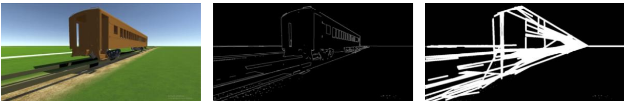
Figure 2: Image of the train created in Unity. Fig. 2A (left) shows the train prior to applying transforms. Fig. 2B (middle) shows the train in Fig. 2A after applying Canny Transform. Fig. 2C (right) shows the train after applying both Canny Transform and Hough Transform.
