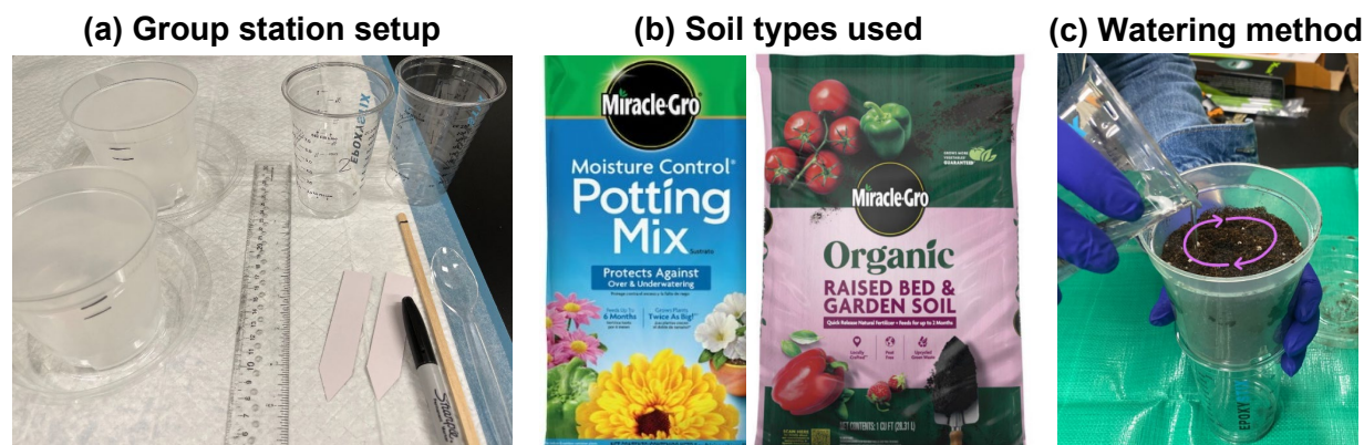
Figure 2: Experimental Setup. (a) Group stations with project materials, including two pots, two measuring cups, two labels, a Sharpie, a ruler, and a wooden stick. (b) Two different soil types used, [Soil 1] and [Soil 2]. (c) The pouring method recommended in the protocol during the flow-through experiment.
