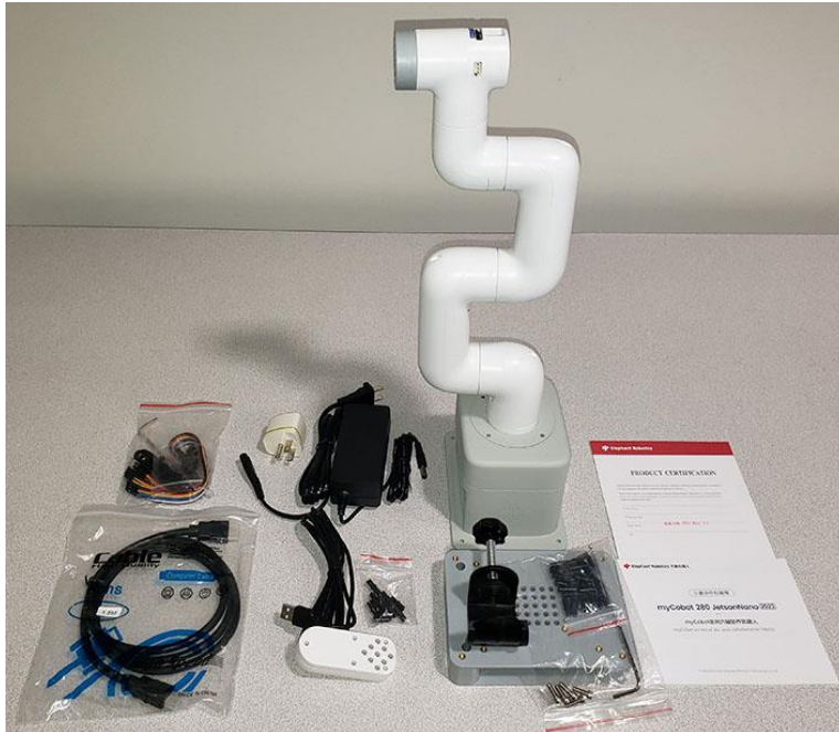
Fig. 1. Elephant Robotics myCobot 280 Jetson Nano Robotic Arm
