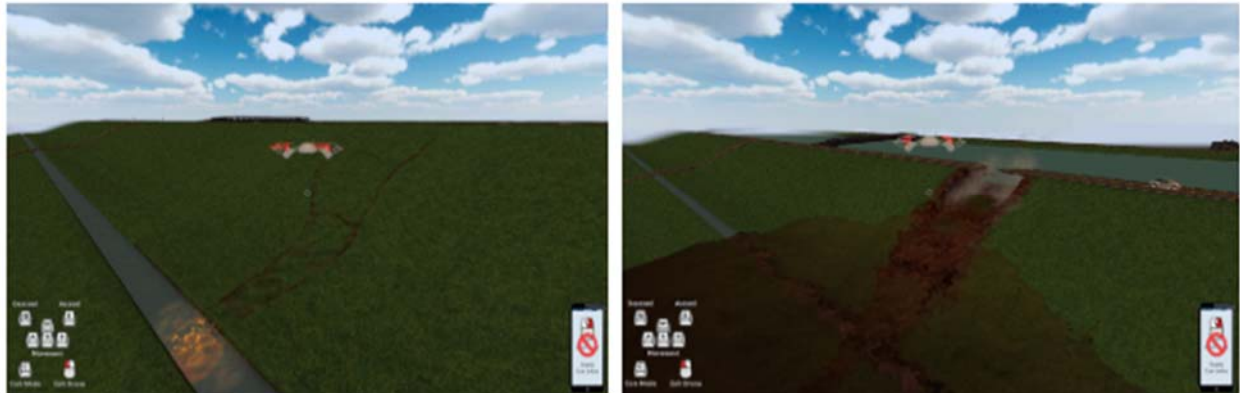
Figure 3: Internal erosion by under piping failure progression in the virtual environment.
