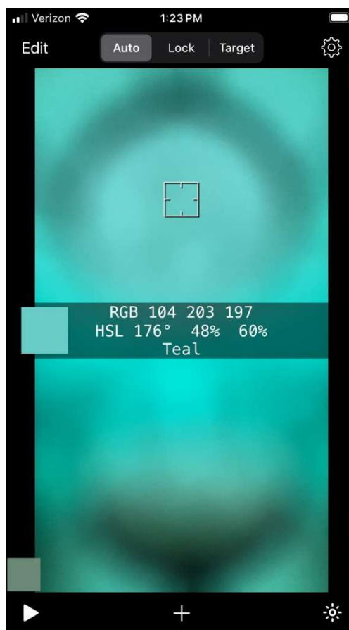
Fig. 2. Screenshot of the ColorAssist Interface used to collect quantitative data. The middle number counts the number of green pixels in the target area on screen which corresponds to the transmittance of green light through the sample.
