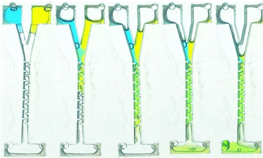
Fig. 5. Demonstration of the module's gravity fed passive mixing mechanism using dye. The module depicted is an earlier version with the component reservoirs set in the middle, relying on surface tension to hold components in place.
