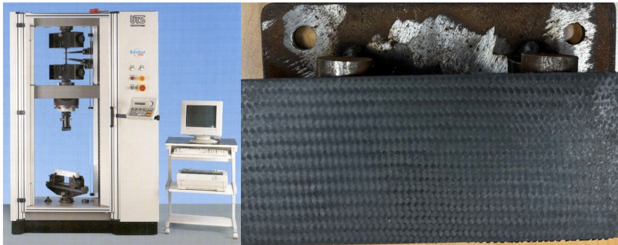
Figure 6. Universal machine and composite plate on support.
