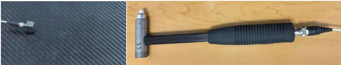
Figure 5. Plate with accelerometer and modal (impact) hammer.
