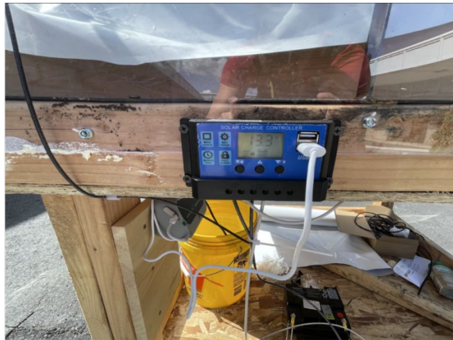
Fig 7. Power produced by the model AGRO-PV Dome as shown in the measurement display of the solar charging controller. The power is used to charge a battery as shown in the bottom floor in the figure
