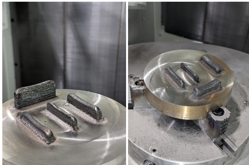
Figure 4 Example test samples during active participation. For reference, substrate diameter is 152.4mm.
