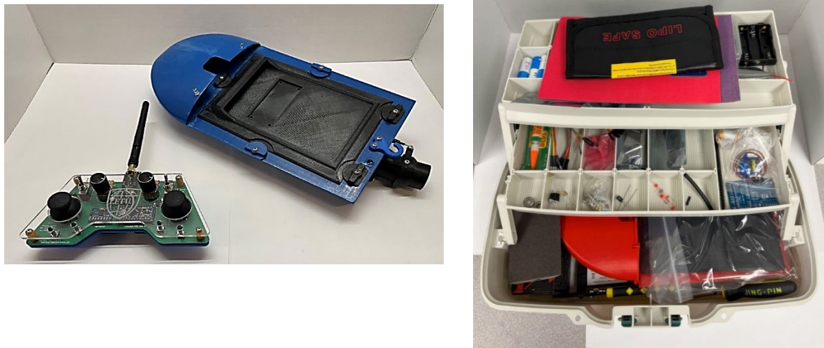
Figure 3: First-Year Build Project: (a) Completed RC boat with Arduino remote, and (b) Initial boat kit provided in tacklebox for storage and transport
