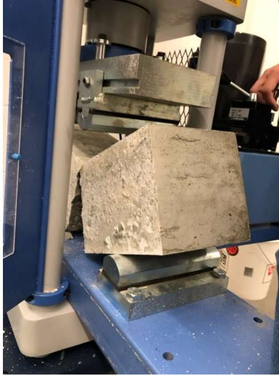
Figure 3: Student Performing Concrete Modulus of Rupture Test
