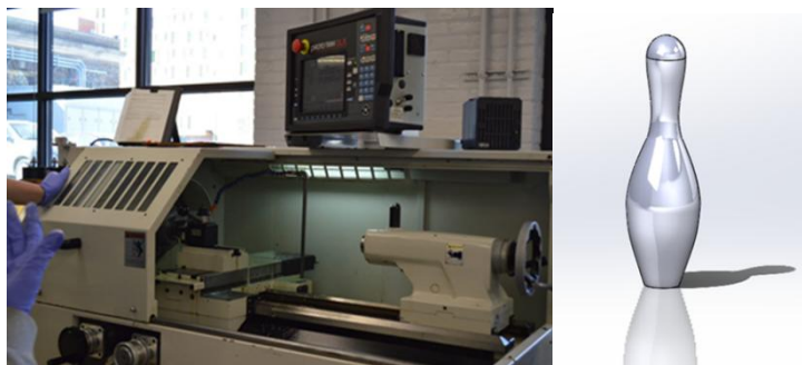
Figure 6 – CNC Lathe and 3D model of bowling pin
