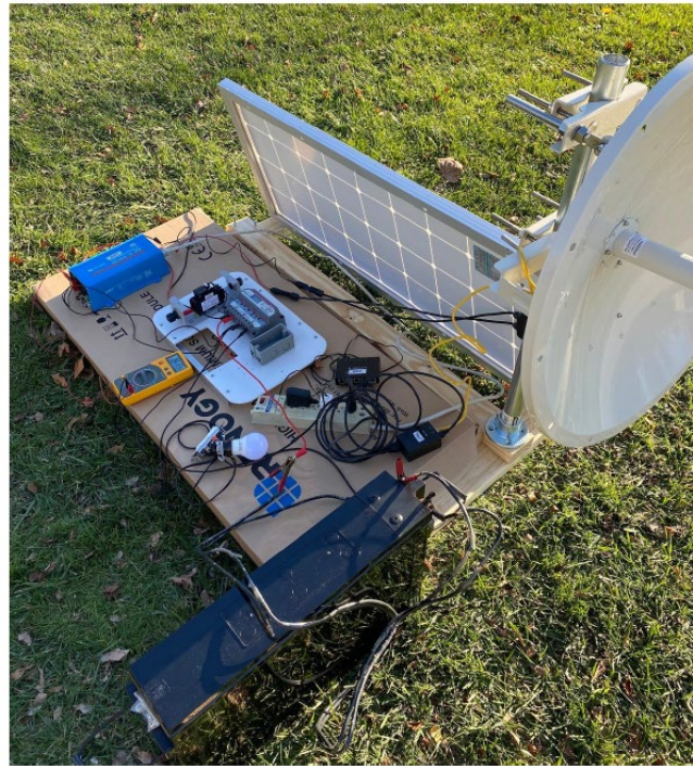
Figure 7. Photograph of Power System Hardware interfaced to networking hardware and dish antenna
