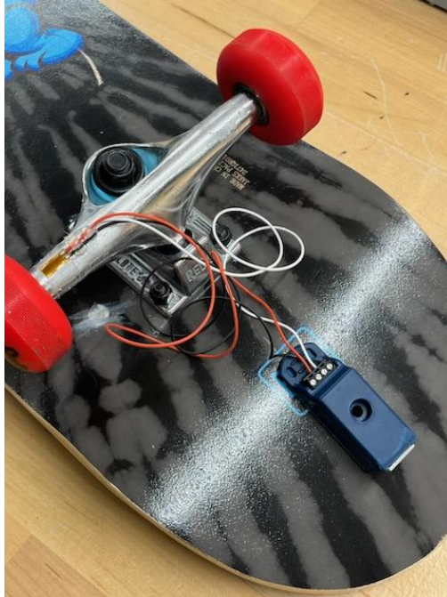
Figure 9– Strain Gage application for LabView Results of Aluminum Truck Deformation
