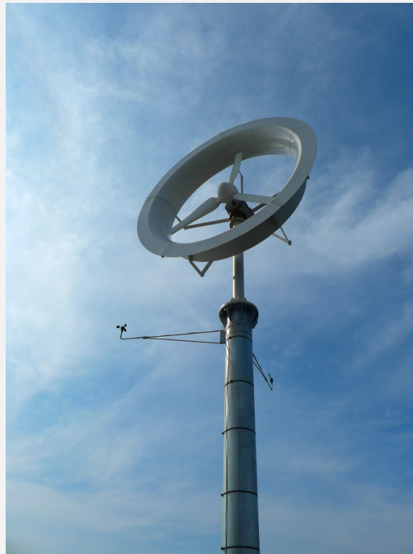
Figure 6: Shrouded wind turbine ("New wind-lens turbine (2012 version)" by Tomon7 is licensed under CC BY-SA 3.0. )
