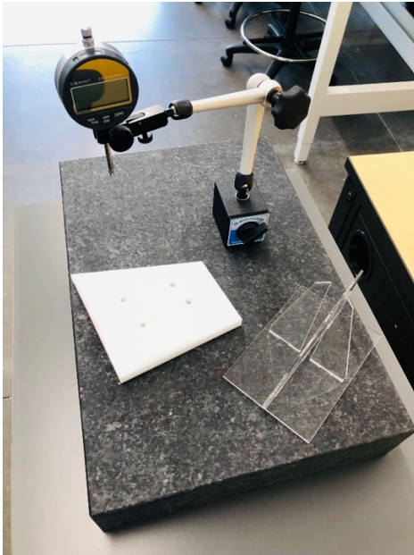
(a) Parts and tools needed to check the angularity of a flat surface
