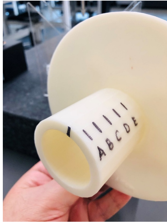
(b) 3D printed part showing the rotation and cross-section guides.
