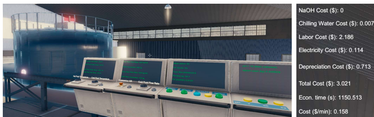
Figure 4. User interface and control panels for operating the photocatalytic CSTR unit in the chemical reactor design VR module (left). Real-time economics analysis feature (right).
