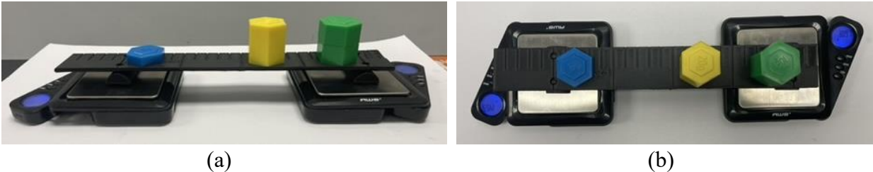
Figure 5. Actual loading set up for equivalent system example (a) profile view and (b) plan view.
