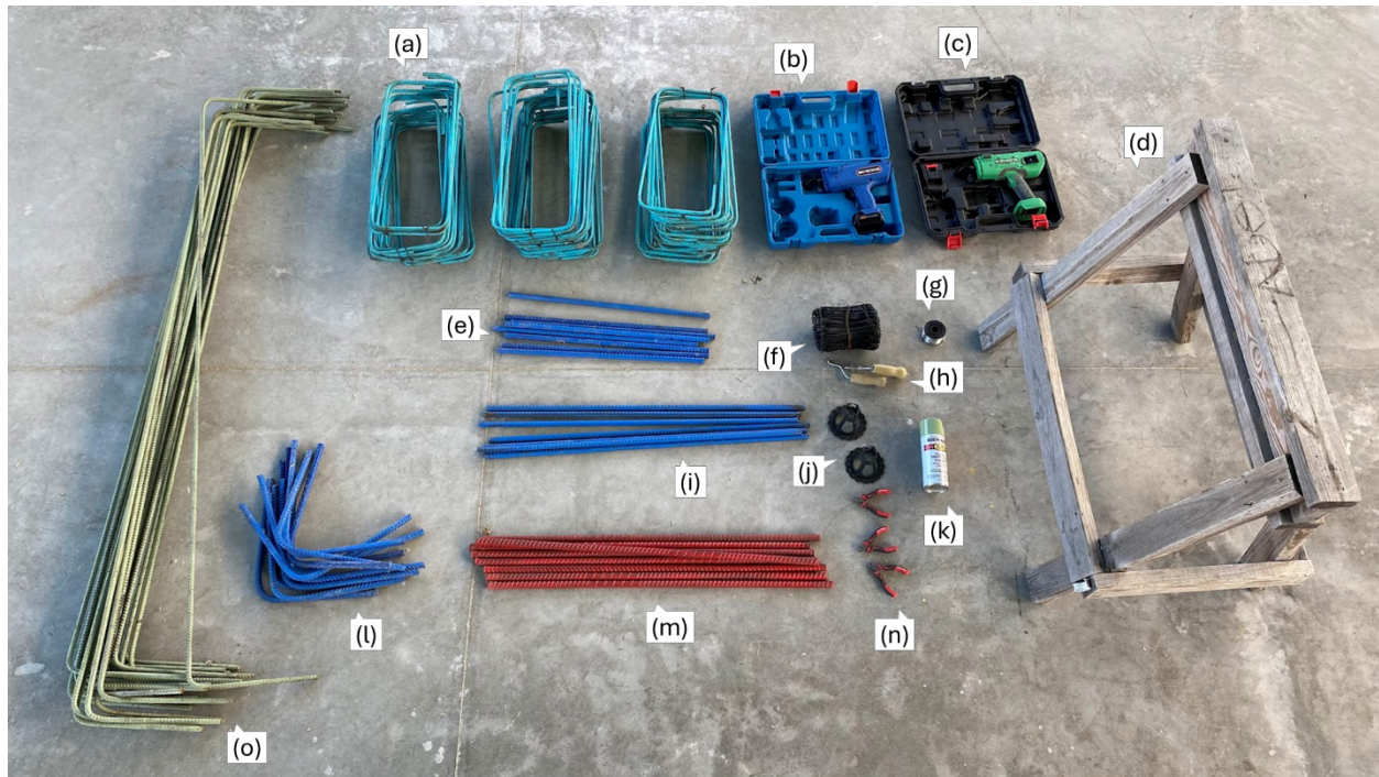
Figure 3. Key laboratory equipment and materials: (a) #3 stirrup 9" x 21", (b) rebar tie gun 1, (c) rebar tie gun 2, (d) sawhorse, (e) #5 straight bars 2' long, (f) double loop rebar wire ties, (g) rebar wire tie coil, (h) wire twister, (i) #5 straight bars 3' long, (j) rebar chairs, (k) rebar paints, (l) #5 12"x12" 90° bars, (m) #6 straight bars 3' long, (n) wire cutter, (o) #4 bars 1'-6"-1'
