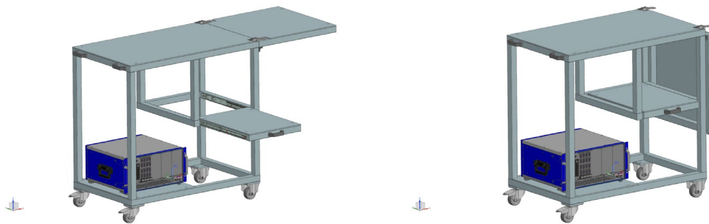
Figure 8: 3D CAD model of the trolley; left in open position, right in transport mode
