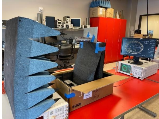
Figure 10 Return loss measurement setup
