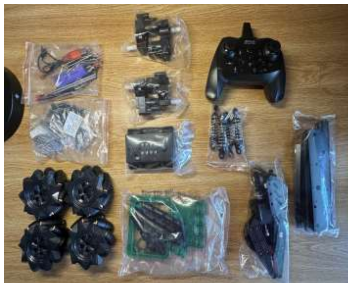
Figure 2: An image of the pieces collected/used in the project. The motors, mecanum wheels, controller, and finger pieces can all be seen. Our Sparkfun kit and 3D printed pieces were utilized as well.
