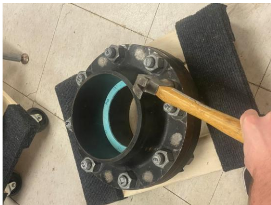
(a) Hitting bolt for flange experiments
