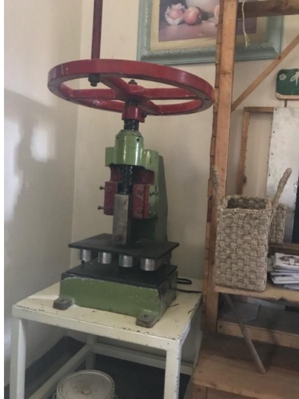
Image 3: This image showcases one of the hand-operated machines used to manufacture sanitary pads.
